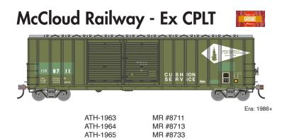
XM class, 50-foot, double door boxcars. Leased 7/1/86 from Itel. Cars in this series numbered 35 in 1987  $^{\ast}$
